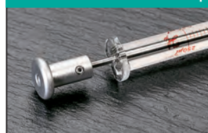
Instrument Plunger CX -Chem with stop TLLX -PTFE Luer Lock with stop
