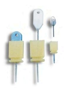
The CMA 7, CMA 8, CMA 11 and CMA 12 Guide Cannulae are coated with silicone on the inside in order to prevent sticking of a dummy or a probe. The guide cannula can be mounted to the stereotaxic instrument using a standard probe clip. Other small items, such as trephine drills and anchor screws are necessary for proper fixation of the guide cannula to the skull.
