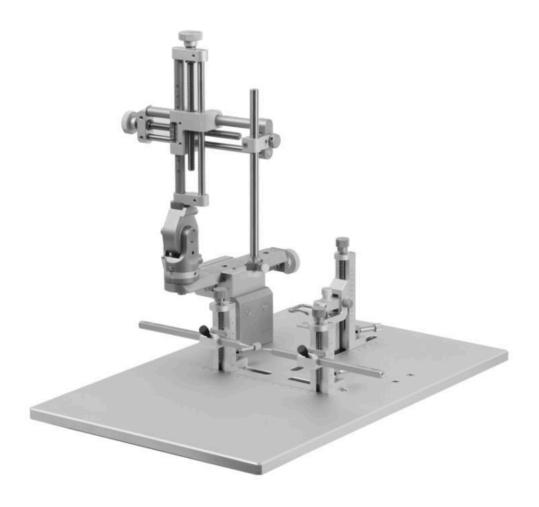
The Harvard Apparatus Digital Compact Stereotaxic Instrument for Mouse and Rat adds a digital manipulator arm with a displacement transducer to the . The compact LCD display allows for real-time coordination presentation of all three axes up to resolution of 10 µm. The display has the ability to run on either AC power or battery power, drastically reducing electronic noise and making it suitable for electrophysiology experiments.
