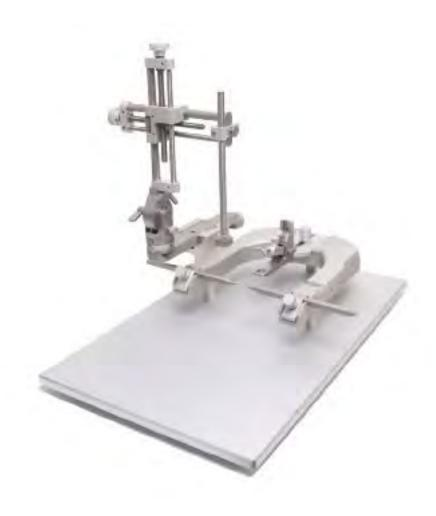
The Harvard Apparatus Digital U-Frame Stereotaxic Instruments add a digital manipulator arm with a displacement transducer to the . The compact LCD display allows for real-time coordination presentation of all three axes up to resolution of 10 µm. The display has the ability to run on either AC power or battery power, drastically reducing electronic noise and making it suitable for electrophysiology experiments.
