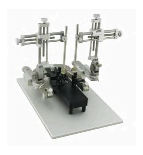
Stereotaxic surgeries can be made simple with the complete Harvard Apparatus Standard U-Frame Stereotaxic Instrument for mouse and neotatal rat. This complete system offers everything you have come to expect in a high quality stereotaxic instrument. The dual-lead screw design ensures stable, accurate and smooth manipulations while the laser engraved scales offer ease of reading. The instrument offers 180° vertical rotation and 360° horizontal rotation, with the ability to lock at any angle.
