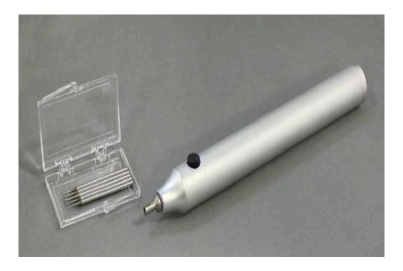
The Ideal Micro-Drill is designed for research applications that require surgical burrs and trephines. The drill is constructed of light-weight aluminum alloy for balance and control and is powered by a rechargeable 6-volt nickel metal hydride (NiMH) battery (charger included). Under normal operating conditions the unit will function for 8 hours between recharging.
