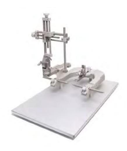
Stereotaxic surgeries on rats can be made simple with the complete Harvard Apparatus Standard U-Frame Stereotaxic Instrument for rats. This complete system offers everything you have come to expect in a high quality stereotaxic instrument. The dual-lead screw design ensures stable, accurate and smooth manipulations while the laser engraved scales offer ease of reading. The instrument offers 180° vertical rotation and 360° horizontal rotation, with the ability to lock at any angle.
