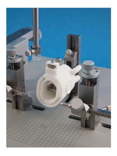
These anesthesia masks for rodent are optimized for different models of Stereotaxic instruments.
