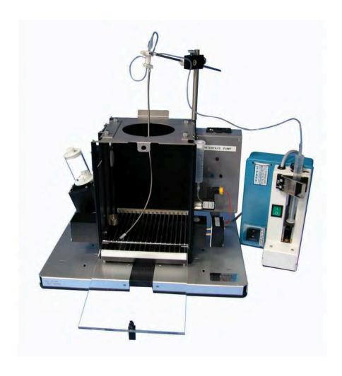
The Panlab Operant Chamber is an entirely modular experimental enclosure designed to conduct operant conditioning procedures (e.g. food reinforcement, DMTS, conflict tests, self-administration…).
