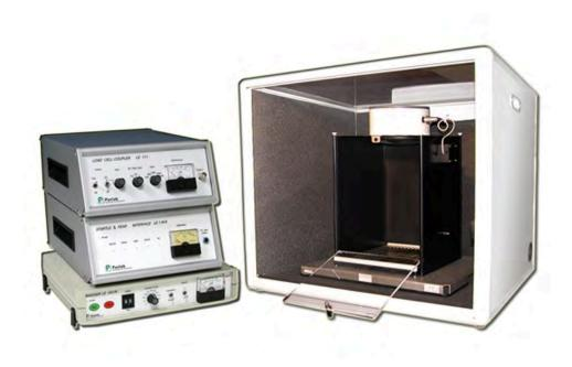
The Startle and Fear Combined system (StarFear system) is a polyvalent system for conducting both fear conditioning and startle reflex experiments in one same enclosure, regardless the animal is a rat or a mouse.
