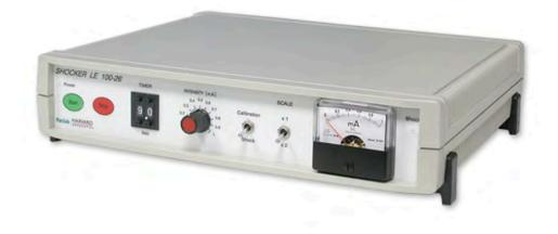
The LE 100-26 is an electric shock generator used in a wide variety of Panlab apparatus for assessing behavior in laboratory animal.
