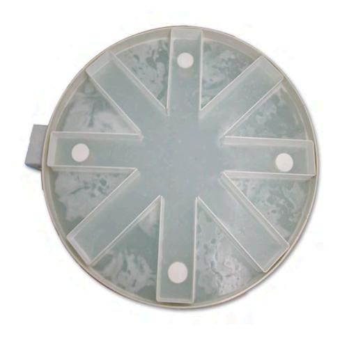
The aquatic radial maze are used for conducting radial maze experiment in a circular pool (water maze). This context is used to avoid any animal deprivation during the experiment.
