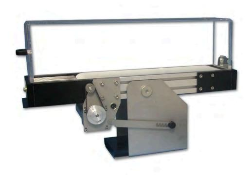
The OxyletPro system is a modular system allowing the integration of respiratory metabolism (O2 consumption /CO2 production). Panlab provides a complete Oxylet solution enabling forced exercise training in a treadmill combined with indirect calorimetry in rodents.
