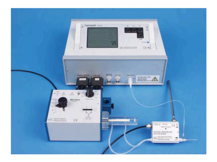
The Type 340 capnograph for rats and mice is equipped with a built-in highly sensitive infrared spectroscopy  $CO_2$  sensor. The sensor is pressure and temperature compensated. The very low volume of the sensor, the optimized system volume and the application of a micro-pump allow very accurate monitoring of respiratory  $CO_2$  concentration on small animals. The Capnograph also includes electronic compensation for interference introduced to signals during  $NO_2$  anesthesia administration.
