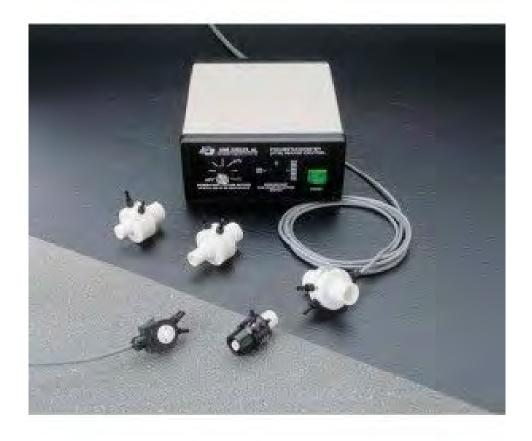
A pneumotachometer converts the flow of gases through it into a proportional signal of pressure difference on either side of a central screen. These Linear Pneumotachometers have a special screen design which assures a linear signal over a range of flow rates and have minimum dead space.
