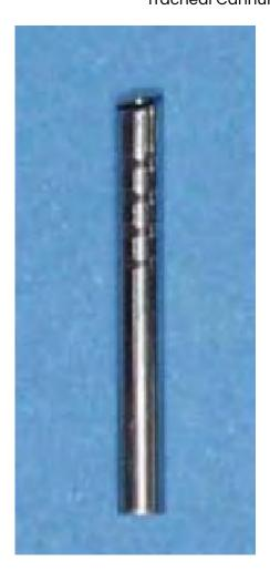
The tracheal cannula is used in a tracheotomy for general ventilation or respiratory mechanics studies. The outside diameter of the cannula must ensure a tight fit to the inside diameter of the animal's trachea.
