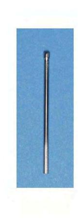
The intubation cannula is used in chronic studies where the animal will be intubated. The outside diameter of the cannula must ensure a tight fit to the animal's trachea.
