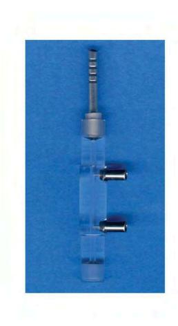
The HSE pneumotachometer PTM is a transducer for airflow measurement on rodents. The main feature of the new design is the small dead space. This ensures a good gas exchange in acute experiments. In combination with the silicon rubber tubing and the tracheal cannula the PTM is used for acute experiments (Intubation or tracheotomy). It is also designed for respiratory flow measurement on isolated lung of rats, guinea pigs or mice.
