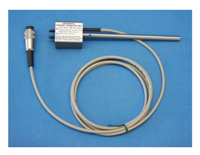
These MPX Differential Pressure Transducers can be used with most research animals to measure tracheal, esophageal or transdiaphragmatic pressures with air-filled catheter. It is ideal for use with mouse, hamster, rat, guinea pig, rabbit, ferret, cat and dog.
