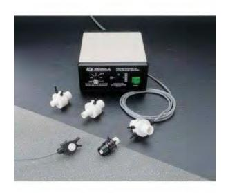
A pneumotachometer converts the flow of gases through it into a proportional signal of pressure difference on either side of a central screen. These Linear Pneumotachometers have a special screen design which assures a linear signal over a range of flow rates and have minimum dead space.
