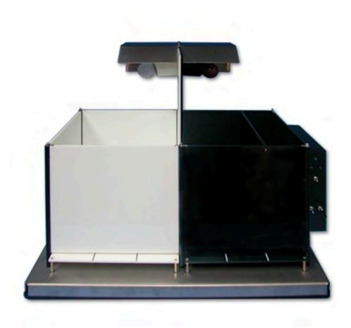
The Panlab black and white (or dark light) box allows easy and quick evaluation of the animal anxious behavior and its modification by pharmacological agents by assessing the animal displacements in two compartments with different size, color and illumination.
