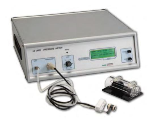
The Panlab NIPB system provides an easy and reliable technique to measure systemic blood pressure and cardiovascular parameters in rodents without invasive catheterization.
