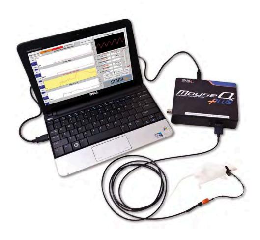
This non-invasive pulse oximeter provides real–time, continuous physiological measurements. It is designed to work with neonatal mice through adult rats. It has a patented design to detect heart rates from 90 to 900 bpm. The MouseOx Plus easily allows researchers to titrate mechanical ventilation and monitor depth of anesthesia.
