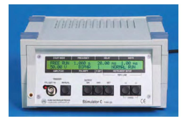
The Stimulator C is a compact, highly stable square wave pulse stimulator that features precise digital timing control. A large LCD display (2 lines at 40 characters) and minimum of controls make setup and operation easy.
