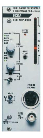
The **Electrocardiogram (ECG) Amplifier Module** (ECGA) amplifies ECG signals. A floating input circuit is used to avoid hum and grounding problems. A bar graph display permits visualization of the ECG signal. The filters are for heart rates up to 1000 beats per minute. Both outputs can be used for recording on a chart recorder or for data acquisition. A square-wave signal generator with amplitudes of 0.3 mV and 1 mV is incorporated for calibration.
