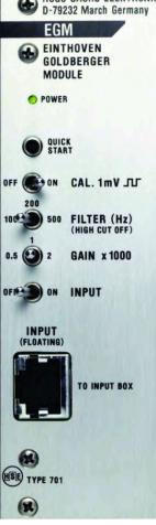
The **Einthoven Goldberger Module** (EGM) is used for capturing and amplifying ECG signals after Einthoven and Goldberger lead configuration in the PLUGSYS system. It connects to 4 electrodes. This module has isolated input amplifiers in order to avoid hum interference.
