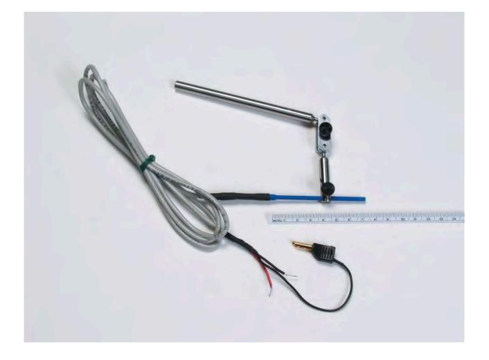
Electrical stimulation of the isolated heart ensures constant heart rate. The tissue is being stimulated between the inner wire and the outer cylinder. Through the coaxial construction, the outer electrode at zero potential acts as a screen so that stray fields are reduced and interference to ECG (EG) recordings is limited. A special holder for easy positioning of the electrode on the heart surface is available as an accessory.
