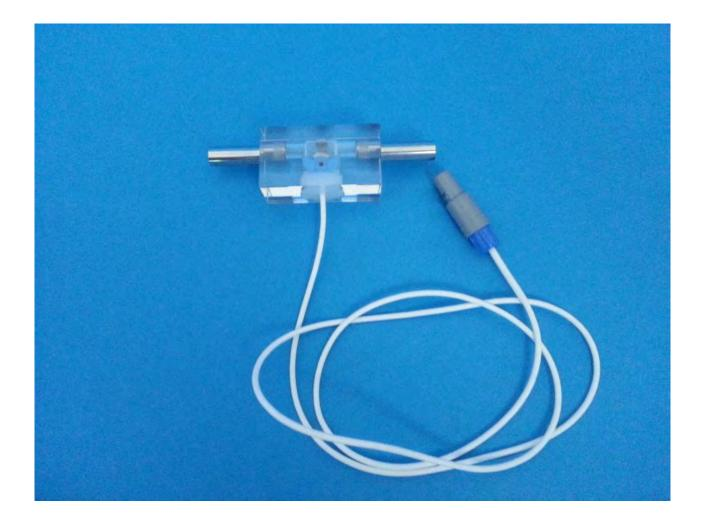
Extracorporeal in-line flow probes monitor perfusion flow on isolated organs. For use with in isolated organ systems such as abdominal organs or lungs, or for any application where a flow in a tube must be measured.
