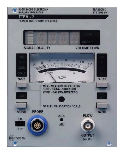
The **Transit Time Flowmeter Module** (TTFM-2) is an ultrasonic transit time flowmeter module used to measure blood flow in-vivo or flow rates of any perfusion solution in isolated organ systems. It incorporates a complete 1-channel Transonic<sup>®</sup> ultrasonic transit time flowmeter which must be connected to a PLUGSYS housing. It can be used either with in-line flow probes or perivascular probes from Transonic.
