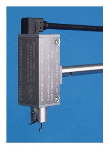
The FT20 and FT50 force transducers are designed for measurement applications in tissue bath experiments where isometric muscle or tissue contraction are measured. The FT20 has a maximal load of ± 20 cN (~20 g force) and the FT50 has a maximal load of ± 50 cN (~50 g force).
