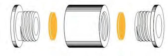
Membranes for ElectroPrep Secondary Link Chambers are available in three membrane materials to suit your application: regenerated cellulose, cellulose acetate, and polycarbonate. Membranes are 7/16" in diameter and precut to fit ElectroPrep secondary link chamber sizes.
