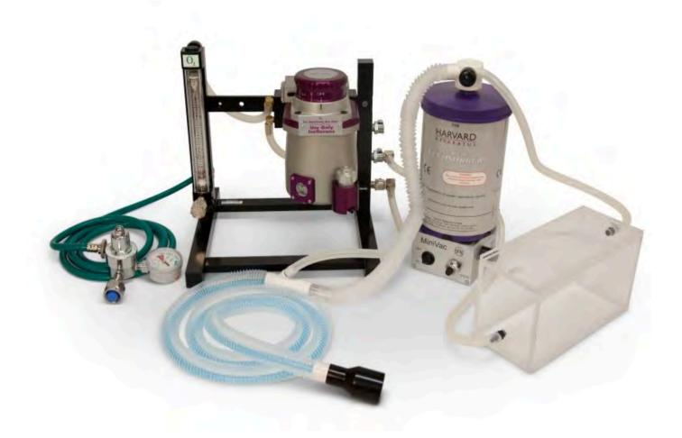
The MiniVac Complete Anesthesia Systems include the MiniVac Gas Evacuation Unit and all of the additional components of a full anesthesia system from regulators, gas hose, and tubing, to vaporizers, flowmeters and nose cones.
