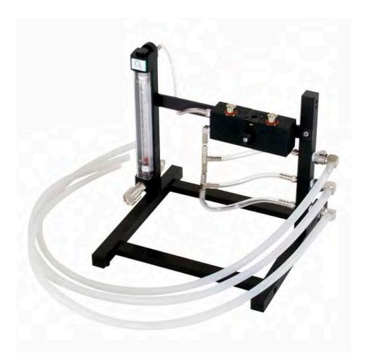
The Tabletop Anesthesia Machine has a single oxygen flowmeter. Its compact design takes up little bench space, is easily portable and can fit into most laboratory ventilation hoods.
