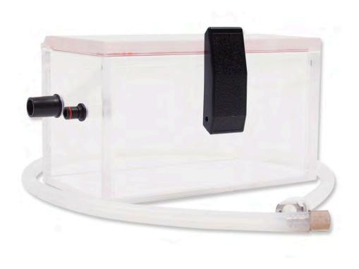
The induction chamber is a very useful piece of equipment that allows you to anesthetize small animals quickly.
